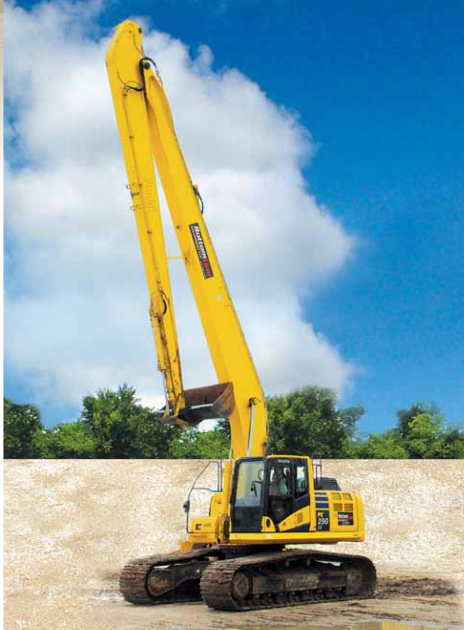
Bottom Line Equipment's fleet includes specialty machines and attachments, such as Komatsu PC290LC-10 excavators with long fronts. It also equips excavators with auxiliary hydraulics to run a variety of attachments.
