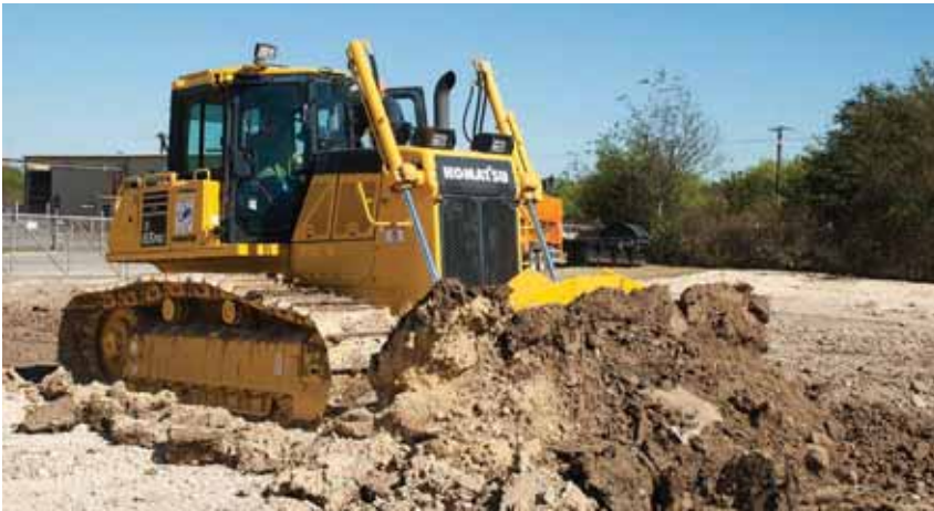
The D65PXi-18, shown at the open house, features fully automatic blade control.
