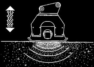
The leader in trench compaction technology, NPK delivers the industry's greatest impulse forces with overall superior performance through hydraulically-operated rotating eccentric action. Greater vibration forces generate stress waves in granular or loose soil material, bringing the soil's air to the surface and packing the particles closer together. Greater impulse action works together with the carrier's downward forces to compact cohesive clay-type soils.
