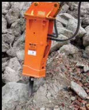
NPK's enclosed hammer bracket option decreases operating noise beyond standard low-noise brackets. Additionally, the enclosed hammer bracket is much narrower than our standard hammer bracket and may be preferred in some trenching applications.
